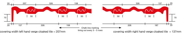
covering width left hand verge cloaked tile = 207mm covering width left hand verge double roll tile = 254mm covering width half tile = 158mm
